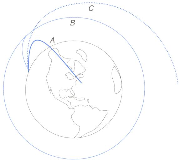
The parabolic path *A* is taken by a space vehicle that falls back to earth. The circular path *B* is followed by a space vehicle sent into orbit around the earth. Path *C*, which may be an ellipse, a hyperbola or a parabola, is that of a space vehicle with sufficient velocity to escape the gravity of the earth and go into orbit around the sun.
